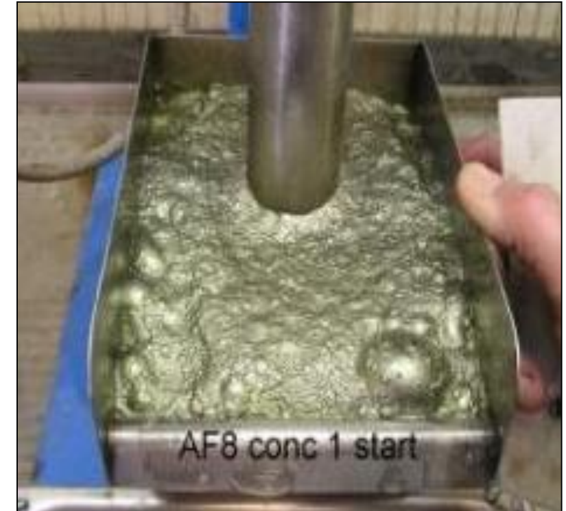
PHOTO: CU FLOTATION FROM WONOGIRI RUN OF MINE ORE
